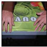
Step 3 Once all corners are inserted, press one silicon edge into channel from corners and work toward the center. Make sure welt is fully inserted into channel. Continue until all sides are done. Smooth out edges of graphic.
