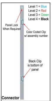
Each component has 2 clips. the lower clip is ALWAYS black. The top clip is color coded to distinguish which level. The color coded clip also contains the numbered label.
