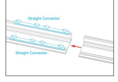
Slide both connectors across seam of extrusions. Tighten all knobs.
