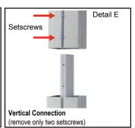
Remove only (2) setscrews when disassembling. Replace setscrews in extrusion after assembling it. Before packing, replace setscrews in extrusion to avoid losing them.
