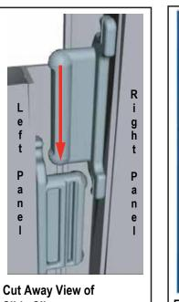
Slide Clips Components connect together by aligning them and sliding downward connecting clips
