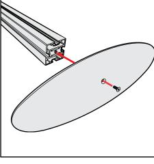
**Base Plate & Extrusion Connection**
