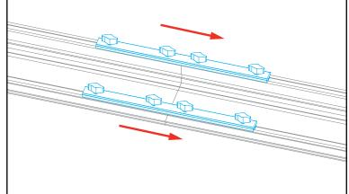
All knobs must be tightened securely to ensure a proper connection.
