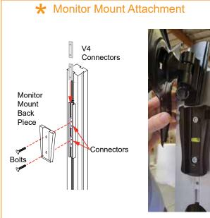
Slide V4 Connectors into groove of Extrusion. Tighten Set Screws to secure connectors in place.
