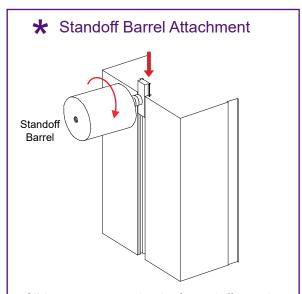
Slide connector on back of standoff barrel into groove of extrusion. Twist to secure in place.
