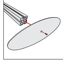
Base Plate & Extrusion Connection
