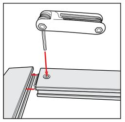
**Extrusion & Lock Connection**
