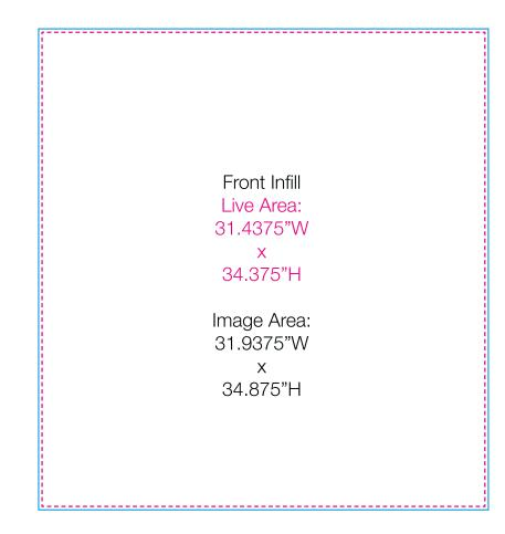
NOTE: 1/4" around perimeter is hidden by extrusion groove
